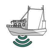
Use sonar equipment to map the ocean floor. Sonar equipment sends out signals that hit the ocean floor and bounce back up to the ship. Then, the sonar machines read the signals that bounce off the ocean floor and create a map on our computer screens.
