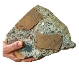
Concrete made with volcanic sand, lime, and water
