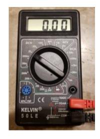
Test the voltage of a battery to make sure the multimeter is working properly. To do this:
