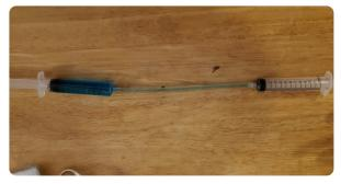
• Create 3 separate Hydraulic Syringe Systems, one for each component of your robot.
