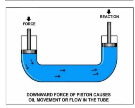
If force is applied to one side of the container, the water cannot be compressed, so the force is transmitted through the liquid. By applying a force to move the piston on one end, the piston on the other end will move the same distance with same amount of force.
