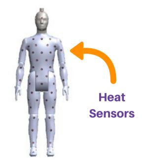
Then, I put the manikin in the testing chamber where I can start a fire but keep it in a safe and contained area. When the testing is complete, the heat sensors send the data about the burns to my iPad.
